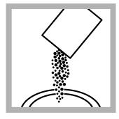
4. Add the contents of one Ferrous Iron Reagent Powder Pillow to the mixing cylinder. An orange color shows if ferrous iron is present in the sample.
