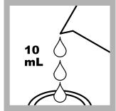
2. Prepare the blank: Fill the sample cell with 10 mL of sample.
